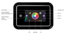
To select the color mode, slide the left wheel up or down until the in mix icon menu is highlighted in the middle.
